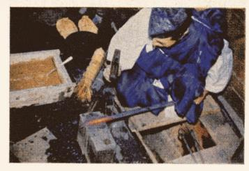
Slender blade is taken from fire and preliminary sharpening of edge is done with file.
