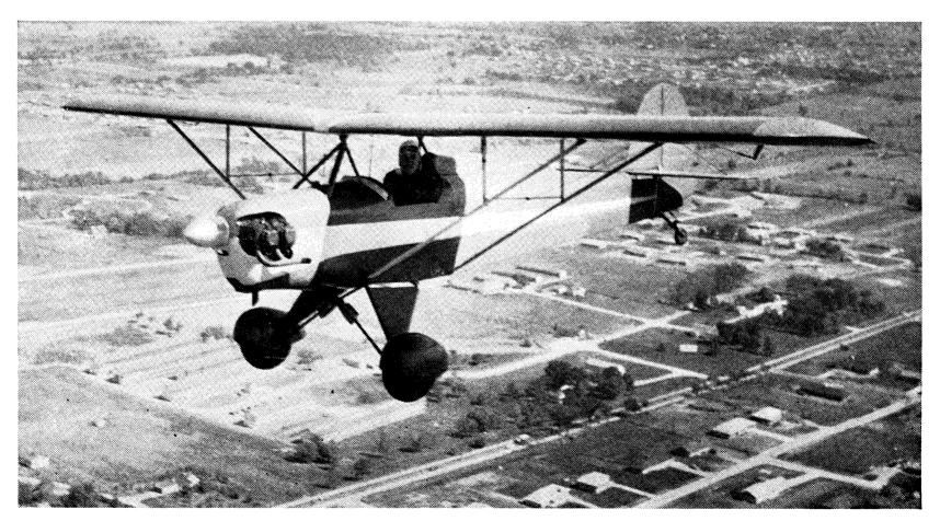
Here Poberezny flies the Baby Ace he built. This plane cruises at 95 mph, can take off in a space of 150 feet.
