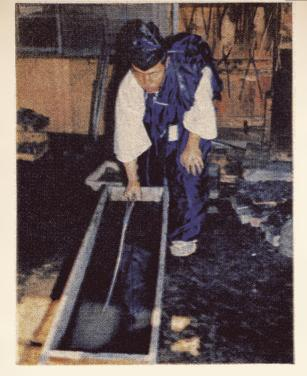
Critical moment comes when blade is doused in water of exact temperature.
