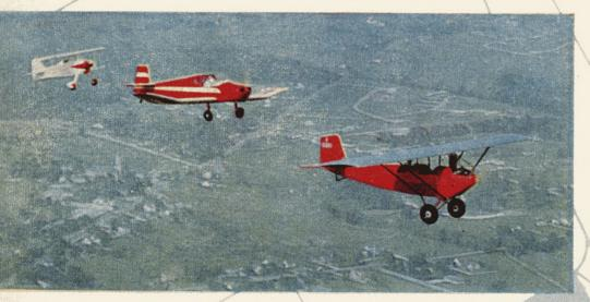
Lead plane is restored Pietenpol "Air Camper," 1930 model, powered by Ford Model-A engine.
