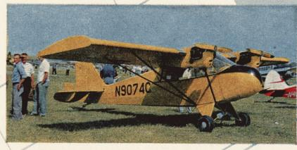
Two 65-hp engines give Irv Miller's "Twin" exceptionally good flight characteristics. Cost to build: \$850.
