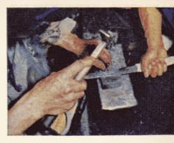
Final step is hammering of hallmark on gleaming blade
